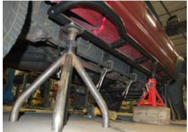
Figure 1. Rock Slider positioned and held in place with jack stands and clamps.
