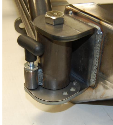
Figure 3. Tire Carrier Pivot Hinge Assembly
