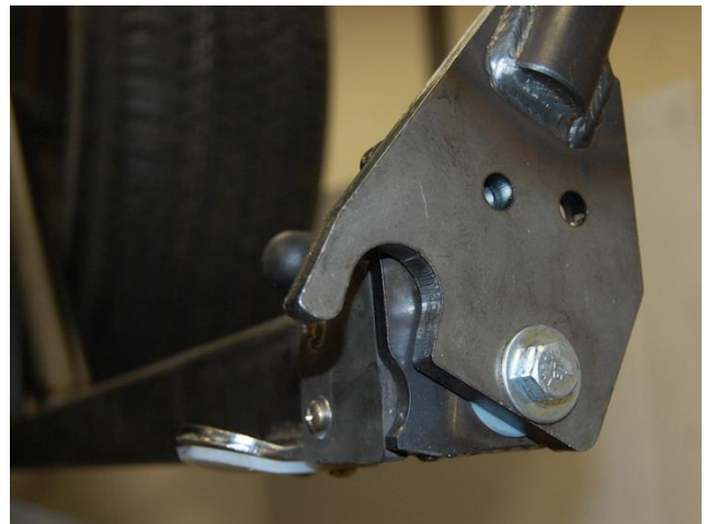
Figure 2. Swing Out Tire Carrier Latch Assembly showing bolt/washer/latch/nylon washer assembly, rubber bumper and nylon latch skid pad.
