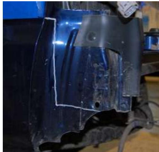
Figure 2. Rear bumper relief cut. Drawn 1 inch lower than first cut should be.
