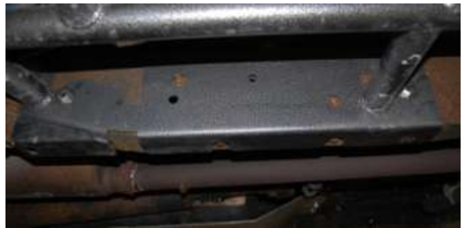
Figure 2. Passenger side rear mount, shown with optional spring skid mount.
