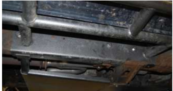
Figure 1. Passenger side front mount. Note it is recommended to use the forward most mounting hole for the front bolt, which requires drilling the side of the frame.
