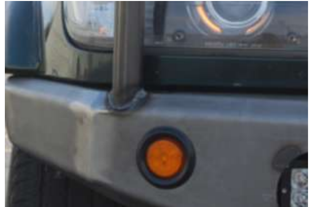
Figure 5. Fully seated turn signal
