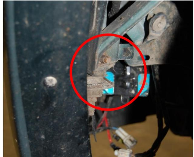
Figure 1. Outer wing bolt backside
