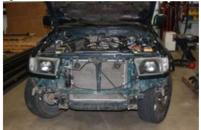
Figure 3. Front bumper removed
