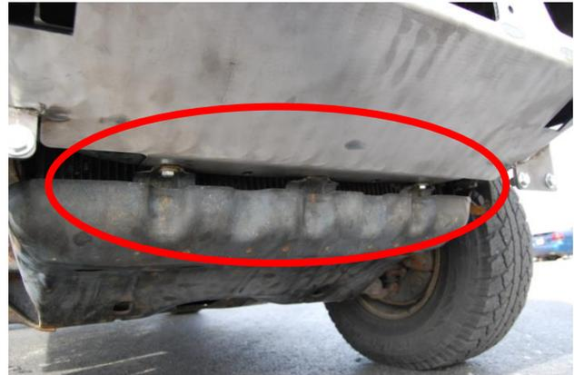
Figure 4. Proper skid plate/bumper alignment
