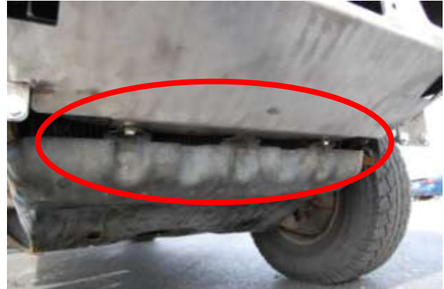
Figure 4. Proper skid plate/bumper alignment
