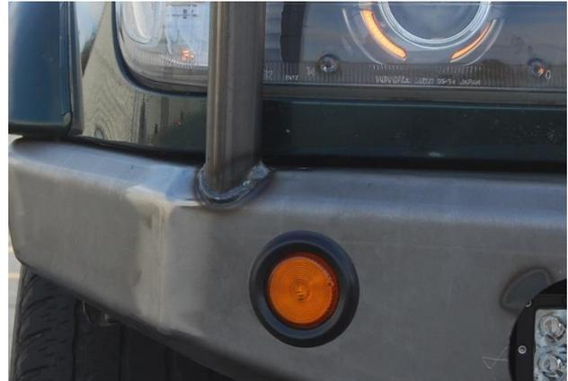
Figure 5. Fully seated turn signal
