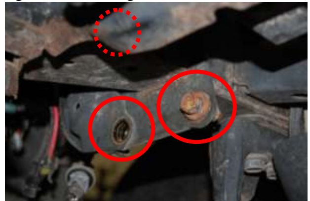
Figure 2. Lower frame horn bolts
