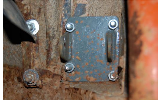
Fig 8 – Lower C pillar mounting plate orientation
