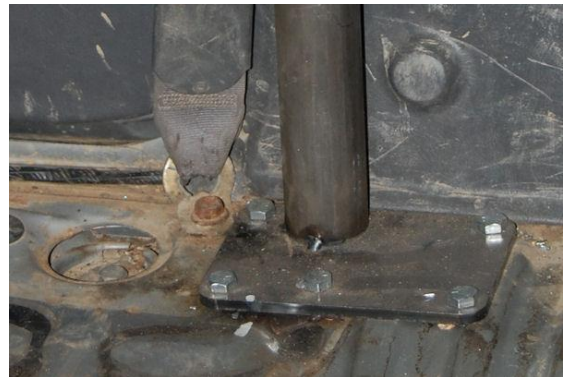
Fig 5 – Upper B pillar mounting plate orientation
