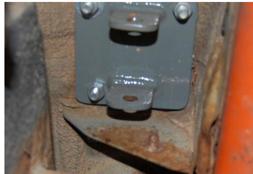
Fig 6 – Lower B pillar mounting plate orientation
